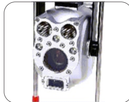
The nose rotates 360 degrees to ensure no dead Angles
